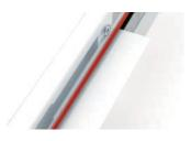
**Cutting line indicator**The red cutting line indicator, which is integrated into the clamp bar, allows precise aligning of the paper to be cut.
